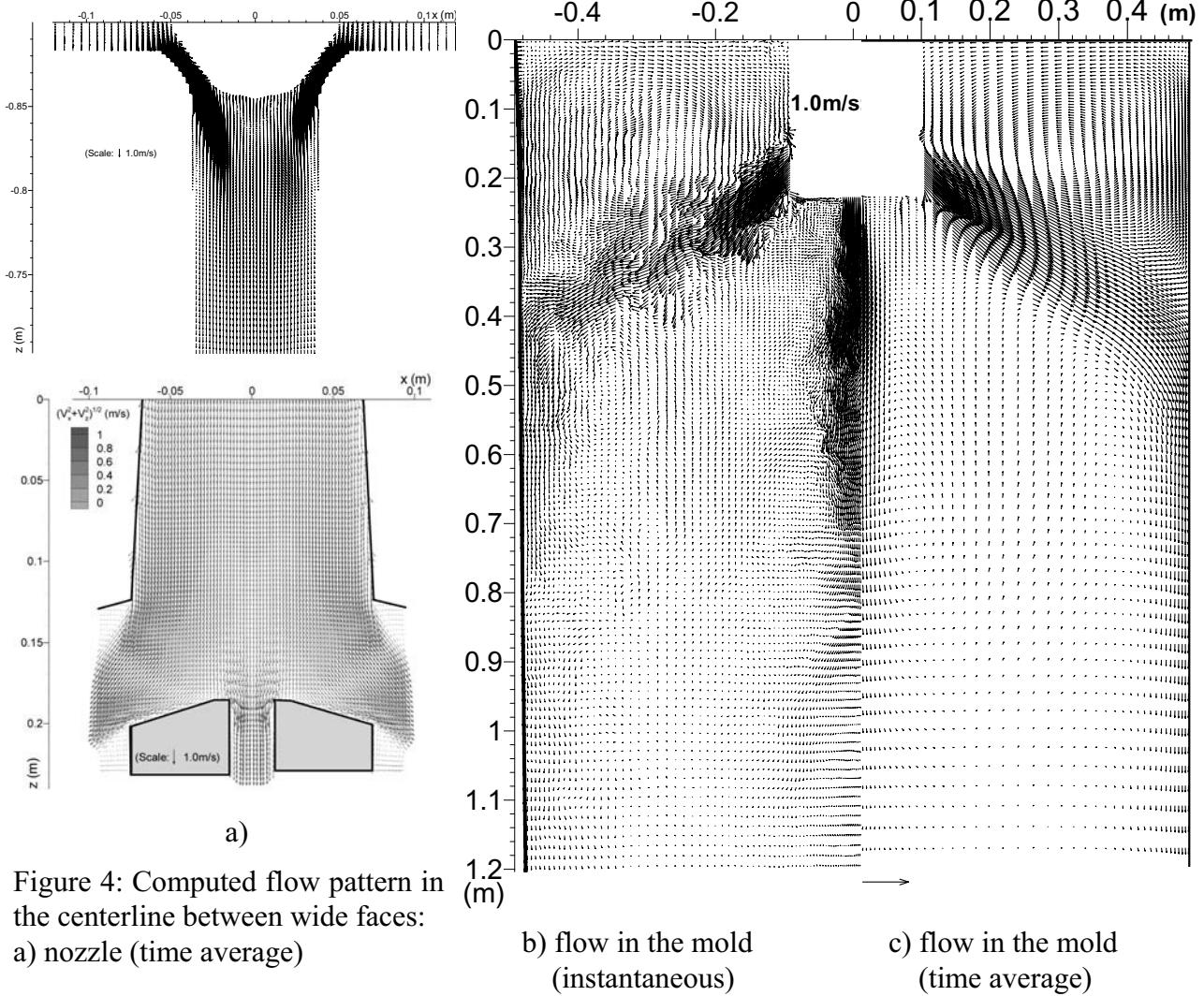
Figure 4: Computed flow pattern in the centerline between wide faces:
